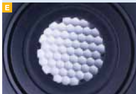
Fly-eye lens for homogeneous fluorescence illumination
