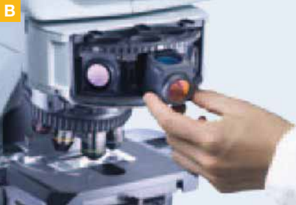
Easy replacement of filter cubes
